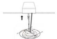
5. Squeeze the V-clips (B) on the back of the disk light and push into open slots on the inside of the recessed housing. Push the disk light upward until flush with the ceiling surface. Note: For wet location applications, apply caulk between ceiling and disk light module.
