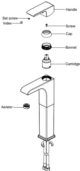
**Problem:** Faucet leaks around aerator or an improper flow pattern.
