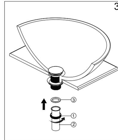
3. Slide the nut (1) over the tail pipe (2). Place the washer (3) into the nut and tighten. Do not overtighten.
