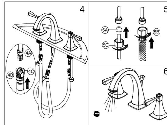
4. Align the tabs (4A & 4B) on the quick connect assembly (4C). Push the quick connect assembly (4C) firmly upward and snap it onto the receiving tube tab. Pull down moderately to ensure the connection has been made. If it is necessary to remove the quick connect assembly (4C), squeeze the tabs on the hose, and then pull down to disconnect.
