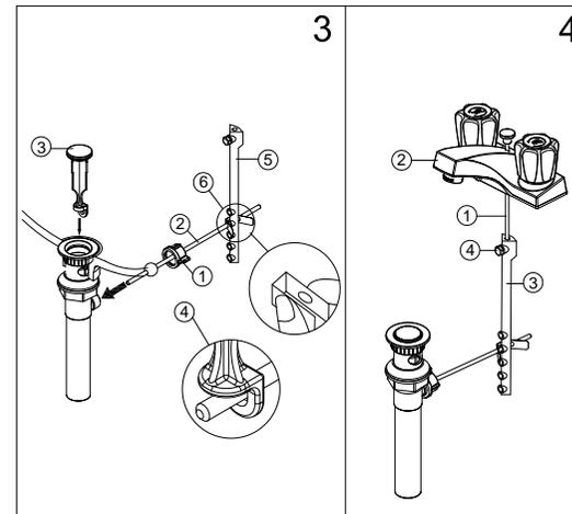
3. Remove the pivot nut (1). Install the horizontal rod (2) and stopper (3), as shown (4). Hand tighten the pivot nut (1). Attach the horizontal rod (2) to the strap (5) using the clip (6).
