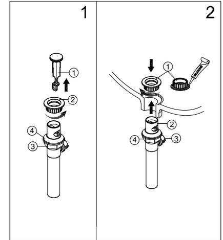
2. Apply silicone to the underside of the flange (1). Insert the pop-up body (2) into the sink. Screw the flange (1) onto the pop-up body (2). The pivot hole (3) must face the back of the sink. Use the groove joint pliers to tighten the nut (4), but do not over tighten. Do not turn the pop-up body (2) while tightening the nut (4) or the sealant may not seal properly. Clean away any excess putty.
