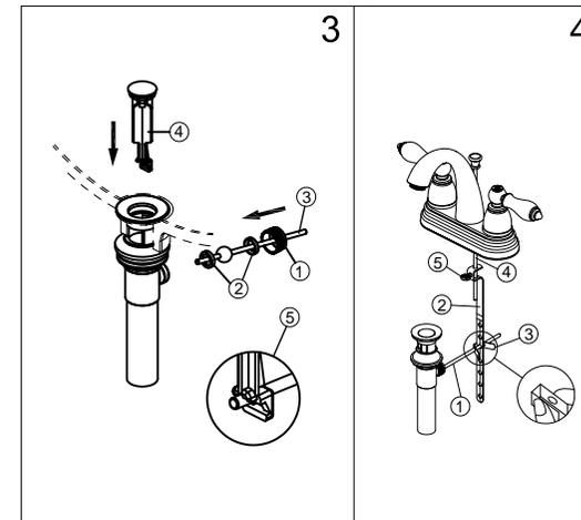
3. Remove the pivot nut (1). Retain the seal (2) on the horizontal rod (3). Install the horizontal rod (3) and the stopper (4) as shown (5). Hand tighten the pivot nut (1).
