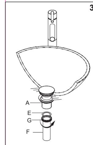
3. Slide coupling nut (G) over tail pipe (F).
