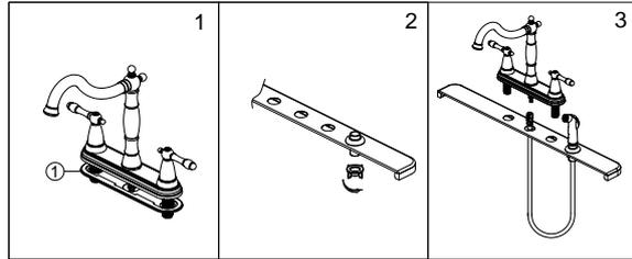
4. Place faucet in position on sink. From under sink, thread mounting nuts onto faucet. Tighten mounting nuts.
