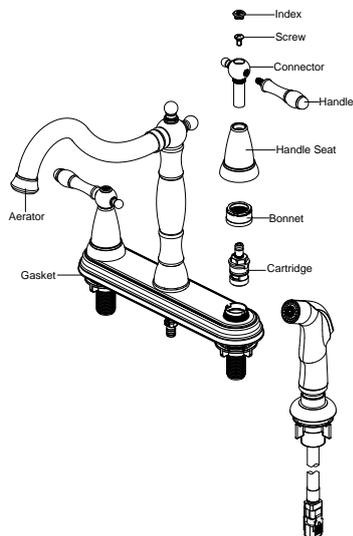
Many of these parts come preassembled. This exploded diagram is to assist in trouble shooting.
